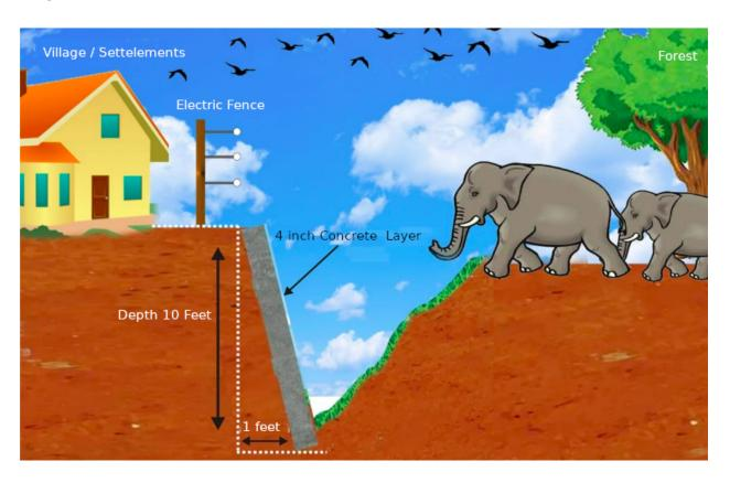
Excavate the existing trench to increase the depth. Reinforce the wall towards the village-side with concrete 4 inches thick to prevent elephants from climbing up.
